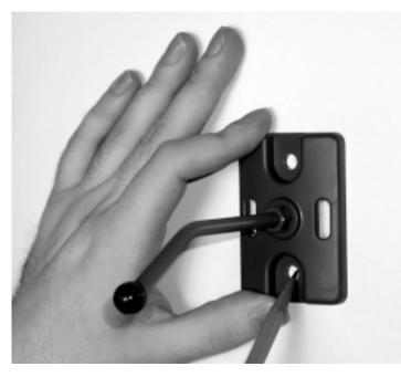
Step 3: Drill pilot holes to keep the stud from splitting at each of the marks on the wall.
